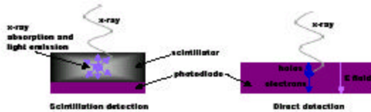
Figure 3 Two possible detection methods: scintillation detection and direct detection
