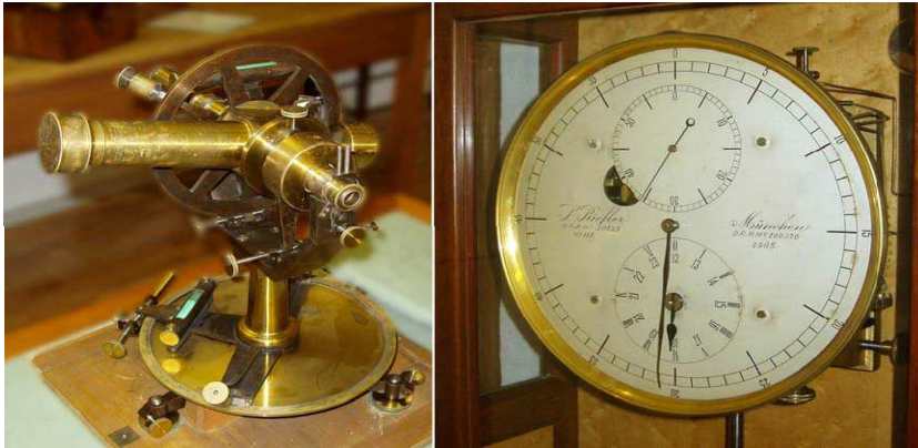
Figure 4. Left : Passage instrument by Eugen-Hammermüller used by Mohorovičić in the period 1892–1913 to daily observe the passage of stars through the local meridian on the Zagreb observatory. This absolute time was recorded by a chronograph, and used to calibrate the Riefler pendulum clock ( right ) which provided time signals for the Wiechert seismographs (exhibited in the A. Mohorovičić Memorial Rooms in Zagreb).
