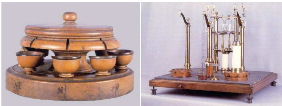
Figure 1. Left : The Cacciatore mercury seismoscope, 1818; Right : The Palmieri electromagnetic seismograph (sensors part), 1856. After Ferrari (1992).
